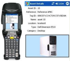
The RFTrack.NET Mobile Audit Module runs on handheld RFID readers and/or barcode scanners. Asset information is synched from the server to a local database on the handheld, allowing users to perform audits and searches even when a wireless network connection is not available.
